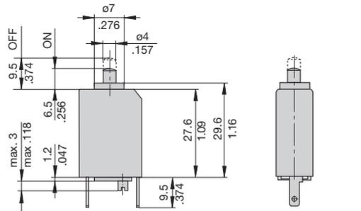
hole for mounting screw M2 usable depth 4.5 mm (.177 in.) blade terminals DIN 46244-A2.8-0.8 (QC .110) cut-out dimensions
