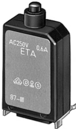
Miniaturised single pole thermal circuit breaker with push-to-reset tease free, trip-free, snap action mechanism (R-type TO CBE to EN 60934) for PCB mounting.
